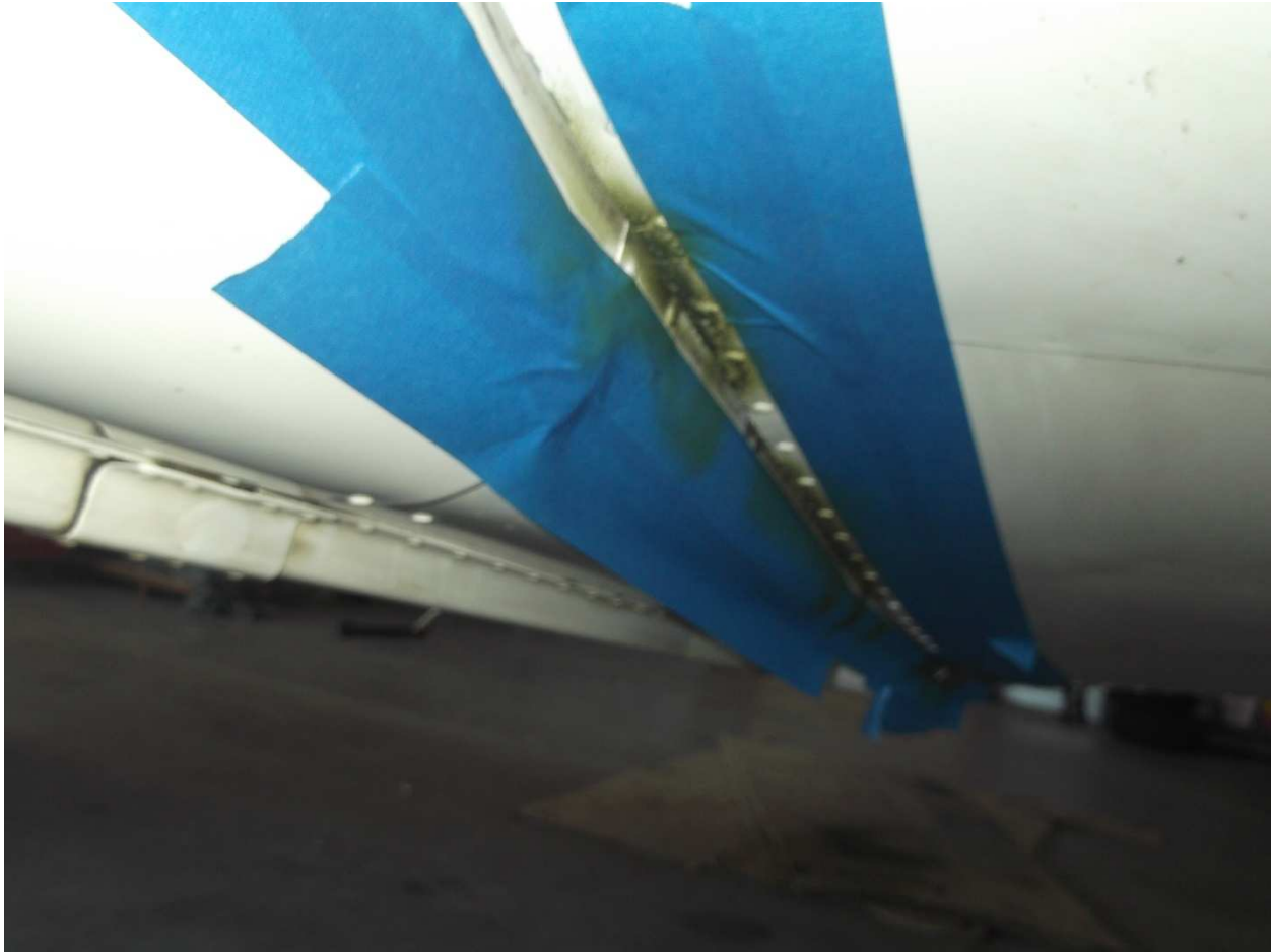
Refinishing some places where the paint had flaked off.
