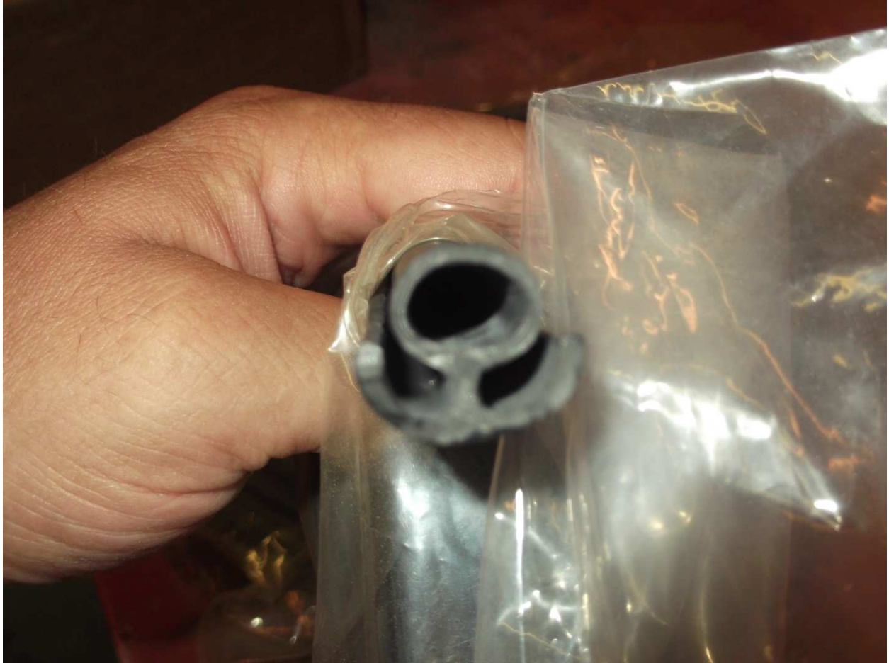
Cross-section of the new wing root seals before installation.
